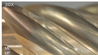
Test 1: Tool wear after 8 hours and 30 minutes of machining
